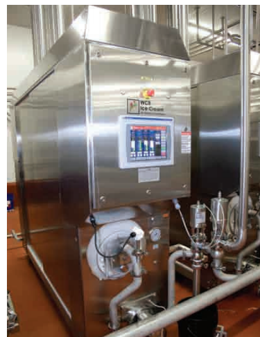
A WCB Anderson hot-melt ice cream carton filler employs an Allen-Bradley PanelView Plus 1250 terminal to monitor, control and display filling rates.
