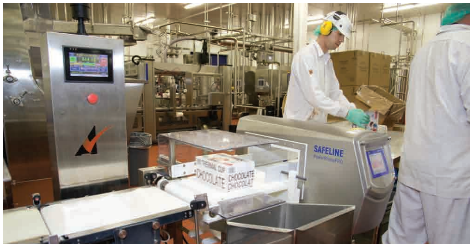
A carton of Chapman's ice cream cups passes through an Alpha Checkweigher and a Mettler-Toledo Safeline PowerPhase PRO metal detection unit, with both units supplied and installed by Shawpak Systems.
