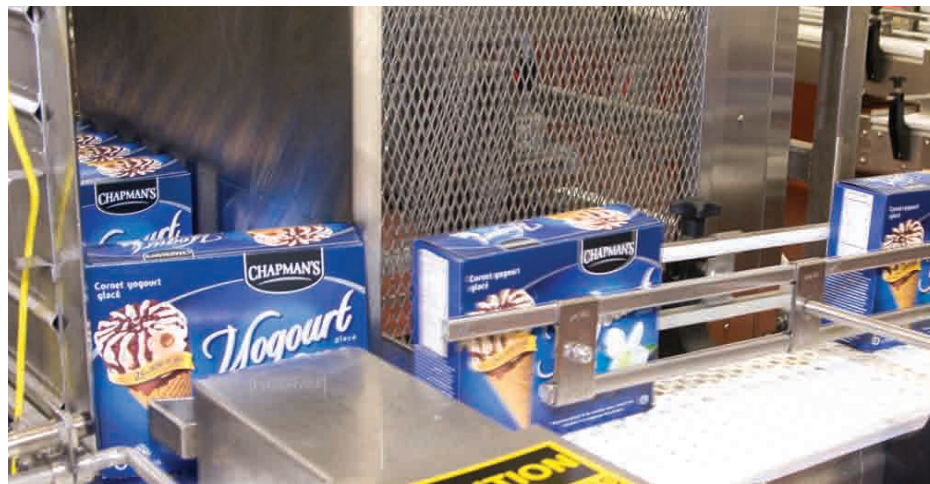
Frozen yogurt products packed in colorful cartons converted by Boehmer Box, a division of CANAMPAC, enter an Arpac 708 E-27 SS shrinkwrapper to be bundled in six-packs for easier palletizing and transport.
