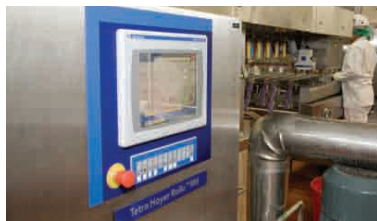
A Tetra Pak Hoyer Rollo RM rotary machine employs Rockwell Automation's Allen-Bradley PanelView Plus 1250 terminal to ensure optimal control over the plant's Lolly line.
