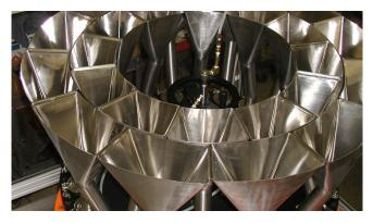
**INNER & OUTER FUNNELS:** Inner and outer funnels make for easy integration with combination scales.
